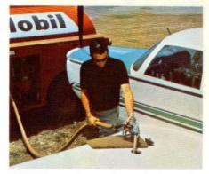
FUELING . . jet-type integral wing tanks are easy to fill. Each fuel cell has a sump drain located under the wing for easy sampling. The sealed, wet-wing tank is easy to maintain and is an added safety feature.
