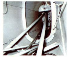
PUSH/PULL CONTROL RODS instead of wire lines and pulleys provide safer and more positive aileron and rudder control and instant response. This feature is the most positive method of connecting the pilot to the control surfaces.
