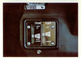
FLAP AND TRIM indicators are located on the center pedestal for easy readout. Trim-ease control wheel at right of pilot seat affords convenient fingertip control.
